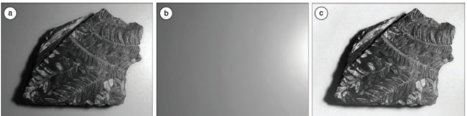
Figure 4.58 Macro image (a) with nonuniform illumination. The background image (b) was recorded under the same conditions with the specimen removed from the copy stand. Subtracting the background image pixel-by-pixel from the original and expanding the contrast of the result produces a leveled image (c).
